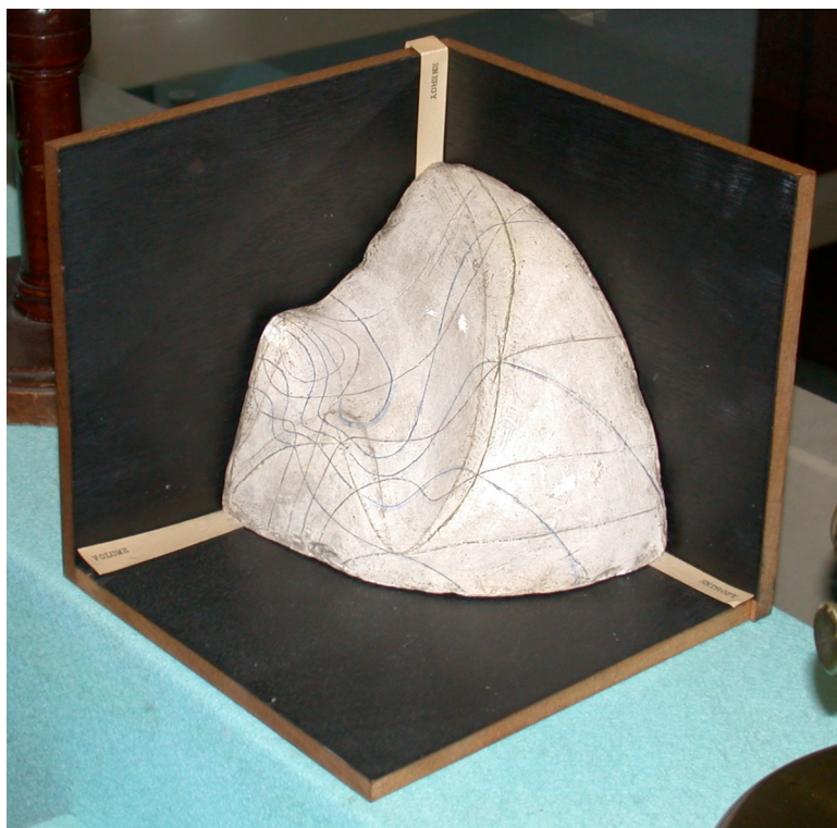
Figure 1. Plaster model of the equilibrium states of water constructed by James Clerk Maxwell and sent as a present to Josiah Willard Gibbs. (© The Cavendish Laboratory, University of Cambridge)
