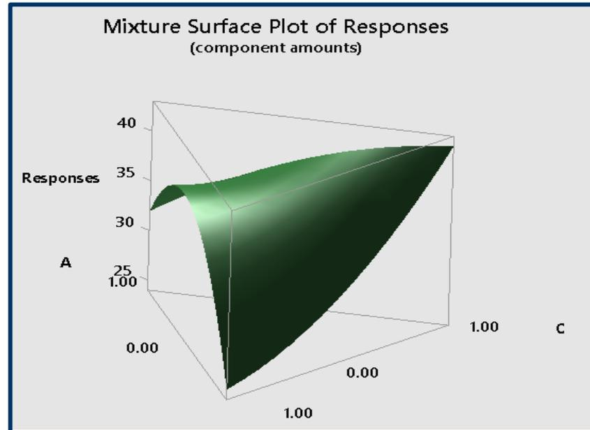
The surface plot (that can be rotated in any direction) provides a more direct representation of the variation of response with the polymer mixture composition, emphasizing the increase in response related to the increase in the percentage of polypropylene (component C).
