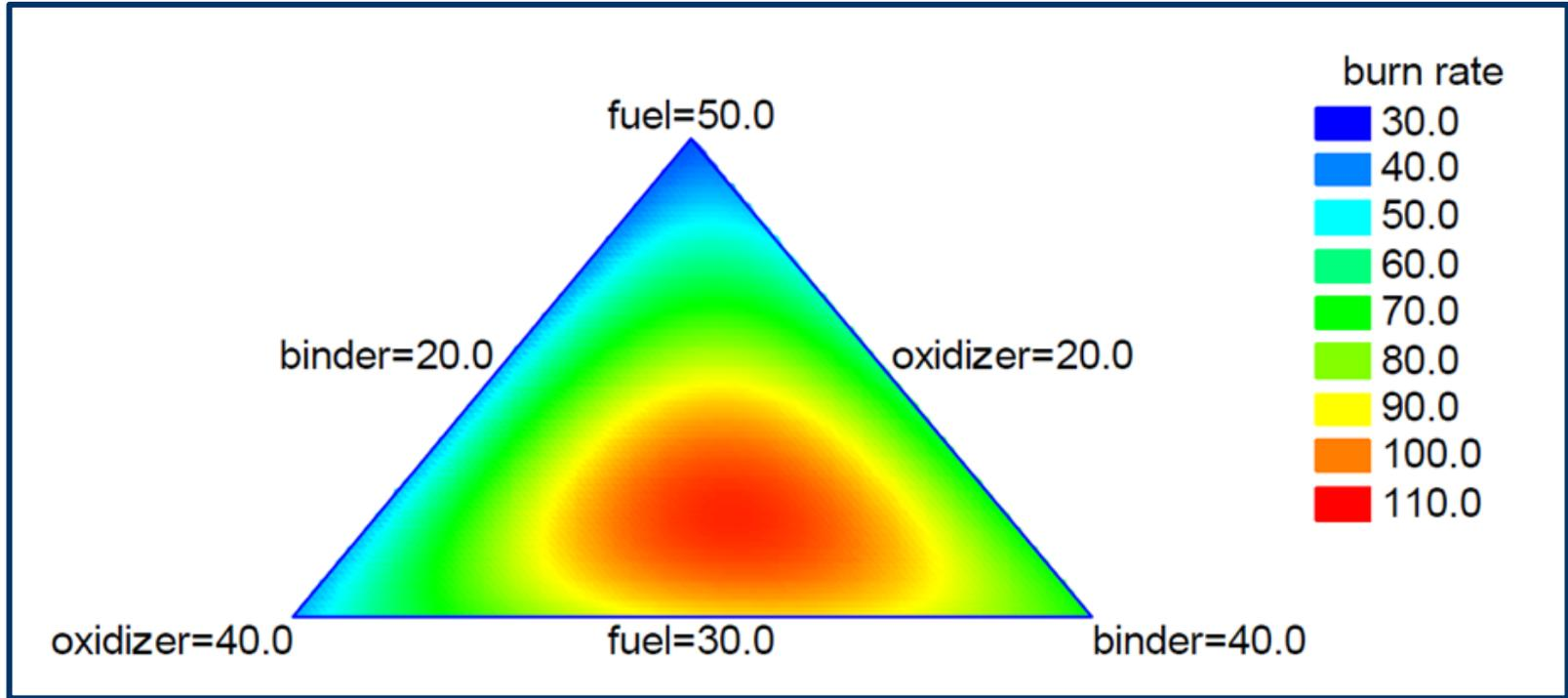
In the table on the right the propellant composition leading to the optimal burn rate, as assessed from the model, is reported:
